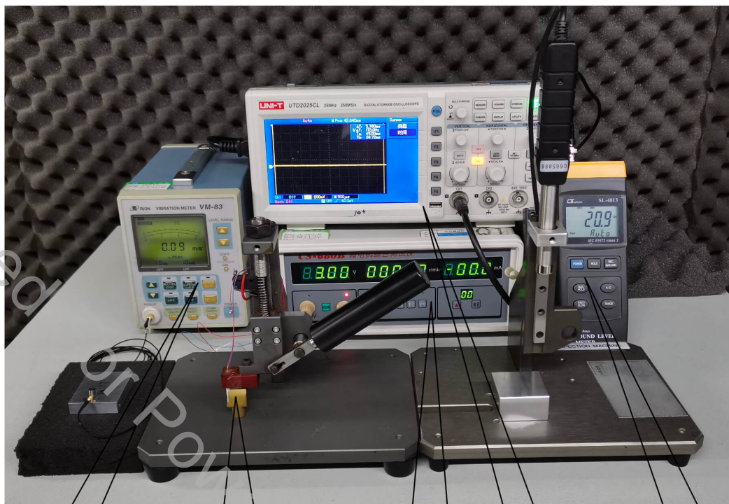
Vibration meter Test Jig (for Clamping the Motor in Place) Multi-functional Test Meter Oscilloscope Noise Test Meter
